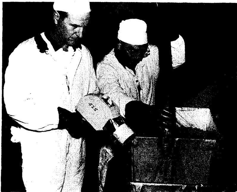
FIG. 22. Boron steel balls being removed from a reactor facility.
