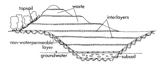
Fig. 1: A schematic representation of a reference dump site, according to (1).
