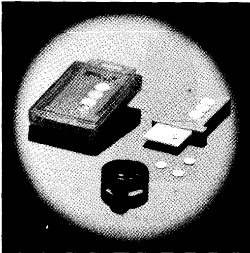
Fig. 1. The Alnor TLD personal badge, dosemeter card and finger dosemeter.
