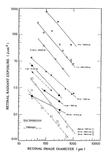
Figure 1. The relationship between the retinal damage threshold (ED $_{50}$ ) and the retinal spot-size.
