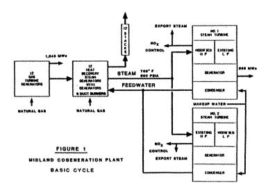
Figure 1 represents a general configuration of the Midland Co-generation Venture that was successful in converting two large nuclear steam turbines into a GT-HRSG combined-cycle arrangement (6).
