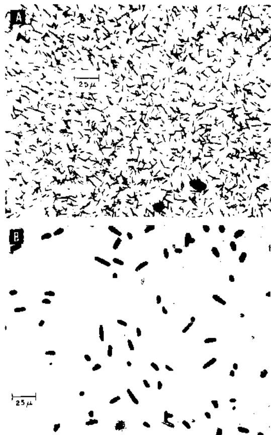
FIG. 5. Fission fragment tracks in Lexan. (A) High track density ( \sim 4 \times 10^8 \text{ cm}^{-2} ) and short etching time (5 min). (B) Lower track density ( \sim 10^8 \text{ cm}^{-2} ) and longer etching time (40 min).
