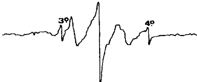
Figure 1. ESR spectrum of alanine irradiated with ^{60}Co gamma rays at 1 kGy 3 .
