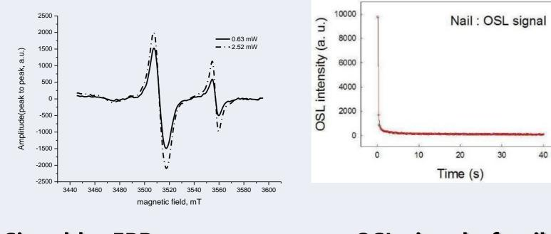
Signal by EPR spectrometer of fingernail clippings at two microwave power level (right : Mn reference, solid rays line : 0.63 Mw, dashed line : 2.52 Mw)
