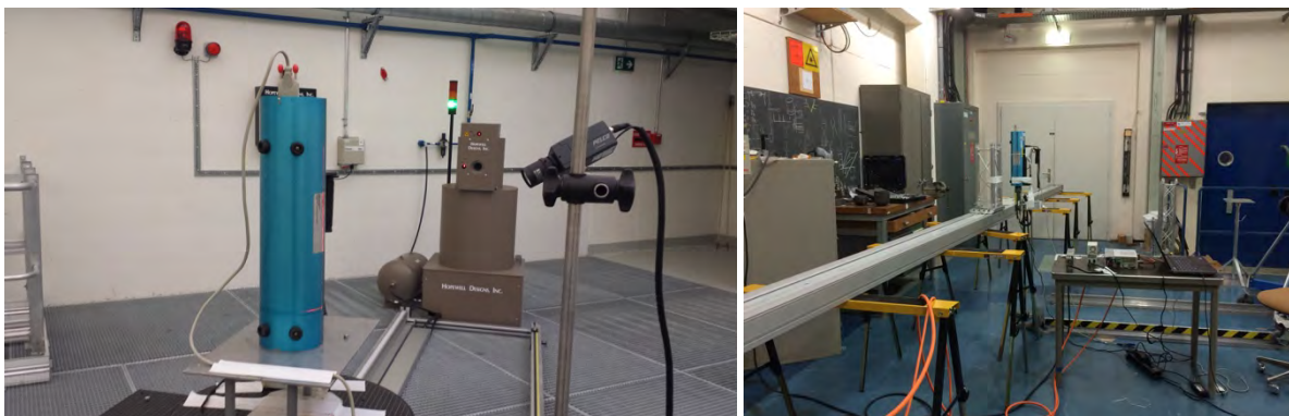
Figure 2: CERN Calibration Facility with irradiator (left) and linear rail test bench (right).
