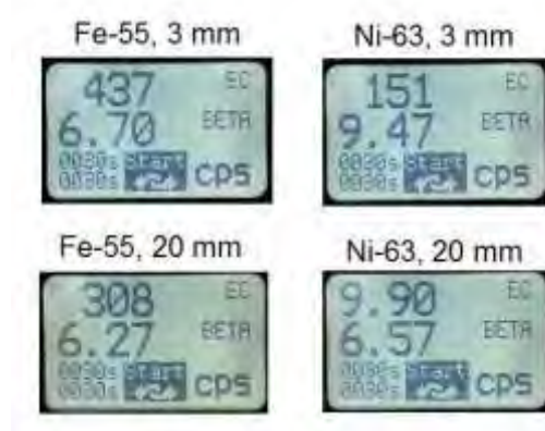
Figure 5: Dual display for Fe-55 and Ni-63 in different distance to the 150 cm 2 source
