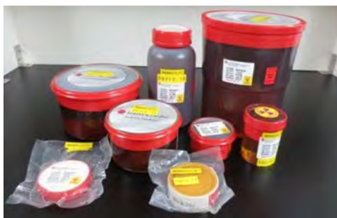
Figure 3: Reference volume sources used for efficiency calibration of the systems. Radionuclides were homogeneously distributed in epoxy resin with a density of 1\text{ g cm}^{-3} .
