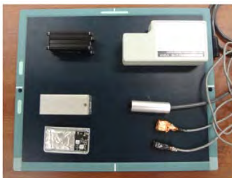
Figure 1: Photographs of detectors. Left upper: iMetry, Right upper:c12137 and Right middle: T-GMK2-S.
