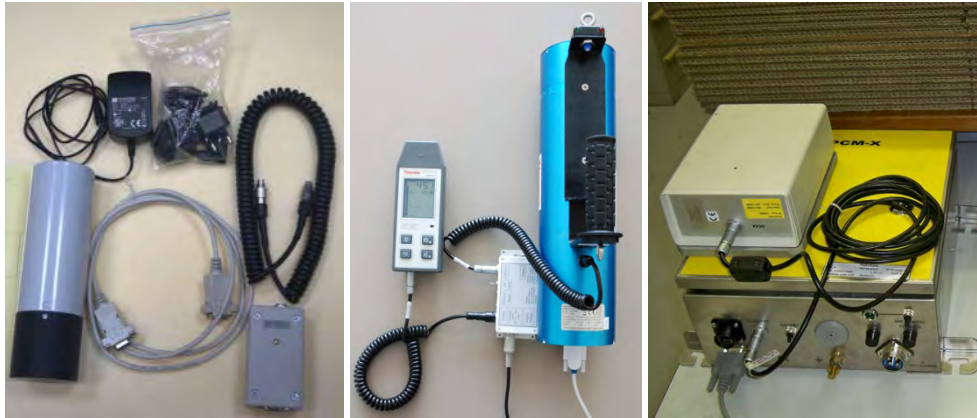
Figure 1: Detectors studied for their suitability to be implemented on the TIM train. Left: ATOMTEX BDKG-24, Centre: Thermo Scientific FH40 & FHZ762, Right: Saphymo PCM-X
