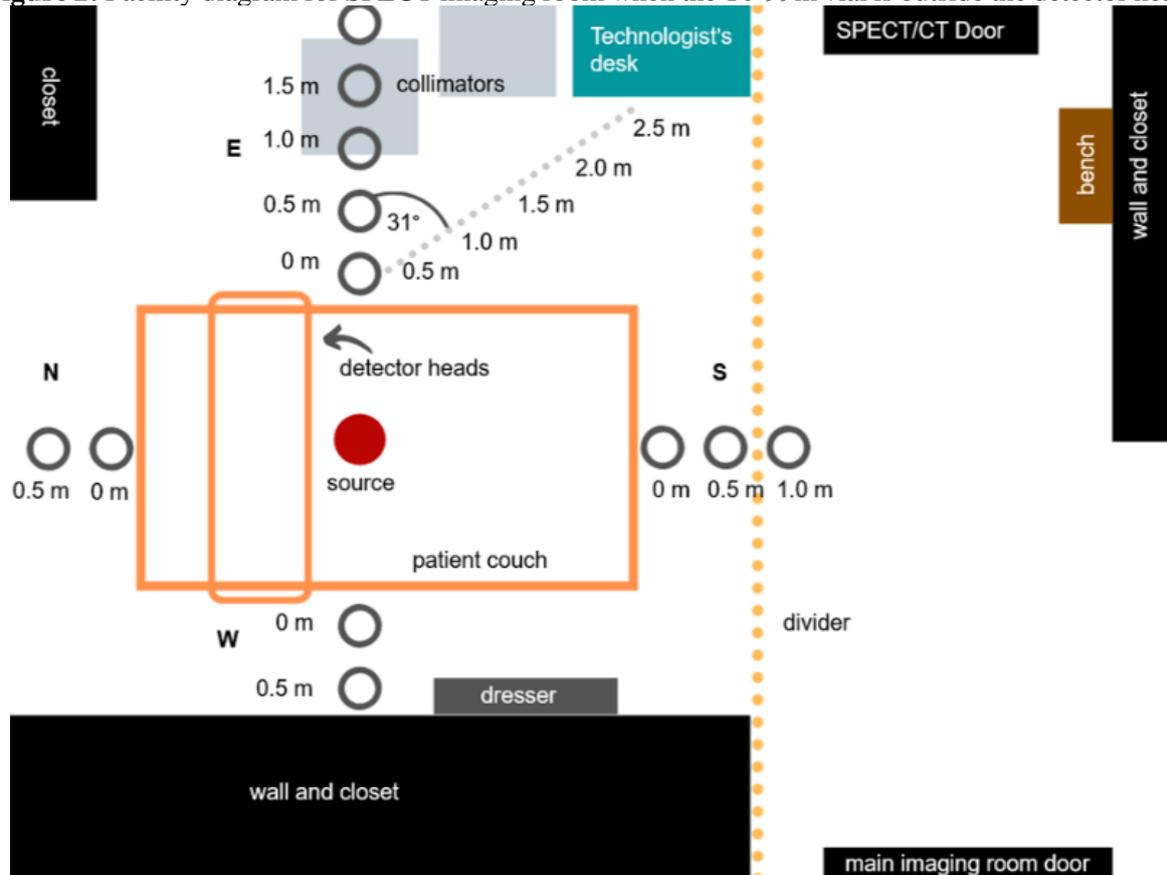
The background radiation level was then measured prior to the actual data gathering using the STEP OD-01 survey meter. This was subtracted to the measured dose rates to get the ambient occupational dose at the said points, which was then used in the calculation of annual dose estimates to the personnel [8].
