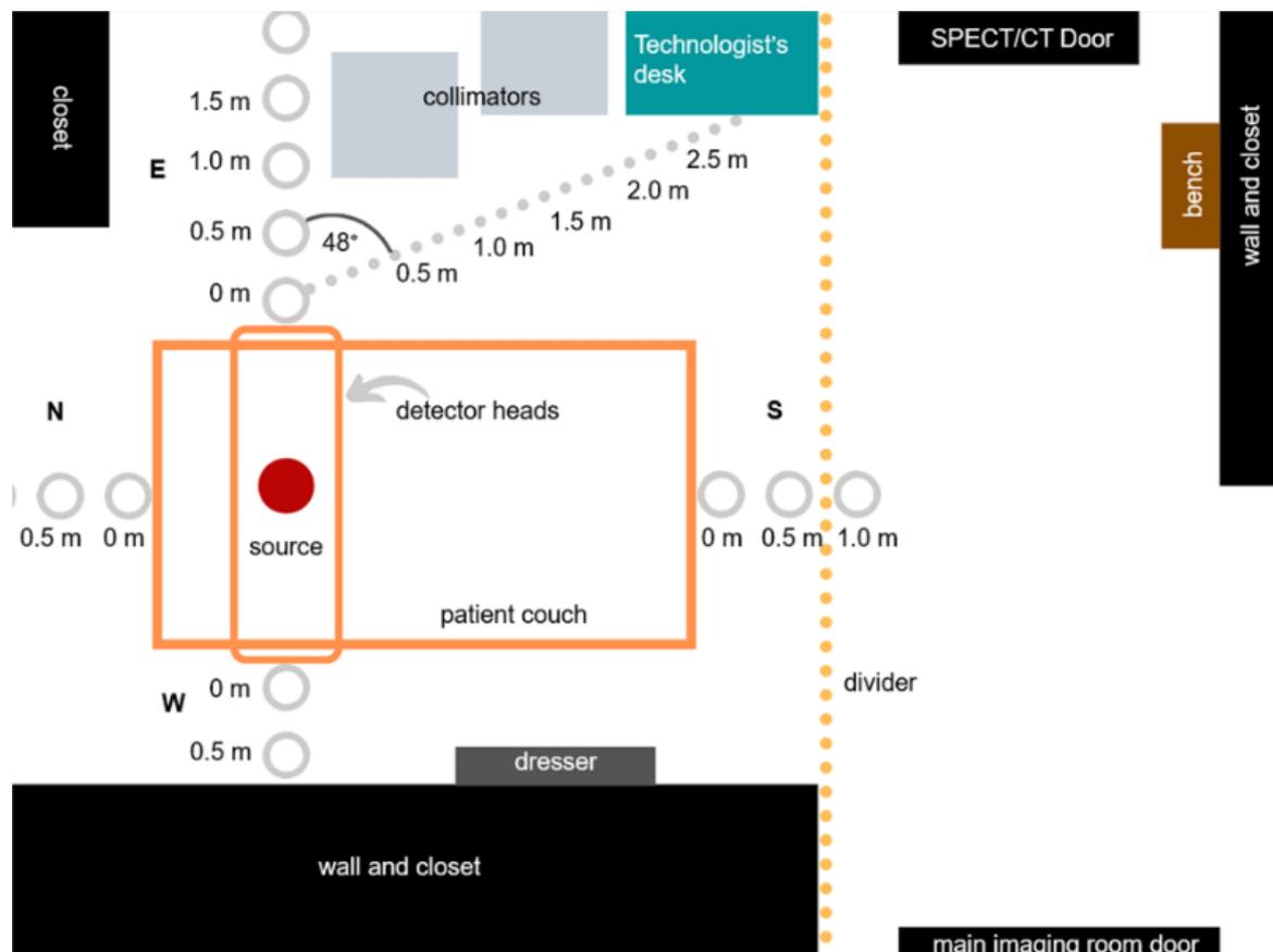
**Figure 2:** Facility diagram for SPECT imaging room when the Tc-99m vial is outside the detector heads
