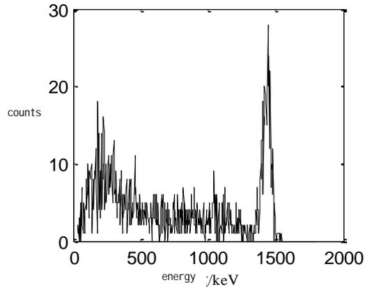
Figure 3.2 Normal gamma spectrum simulated
