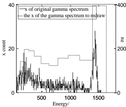
Fig .4.1 Gamma spectrum before and after the site reclassification
