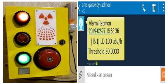
Fig. 8. Indicator of Radiation Early Warning System of RWI.
