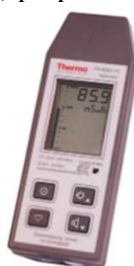
Figure 3: FH-40G (Thermo Fisher Scientific) proportional counter
