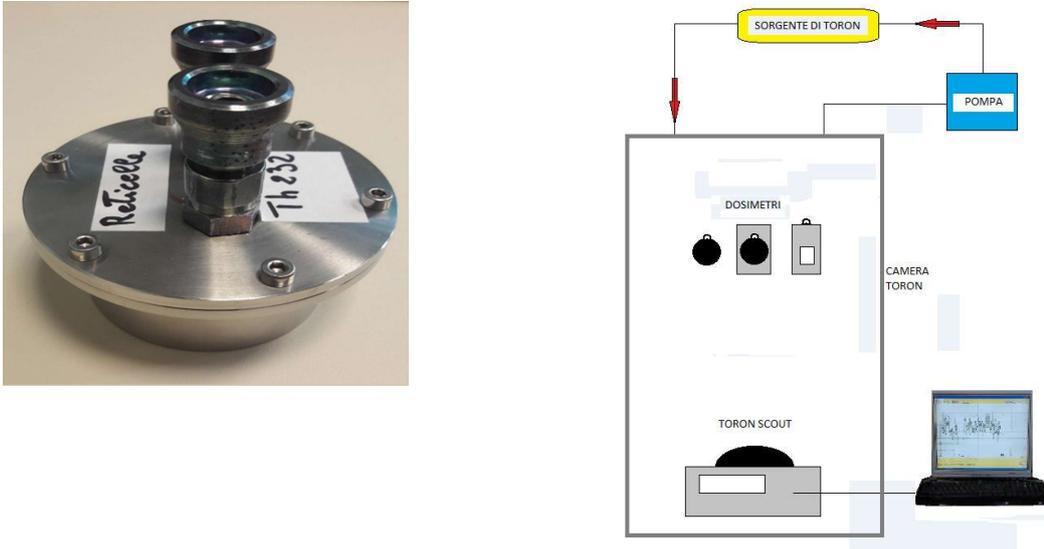
**Figure 4 - The thoron chamber and the experimental apparatus**
