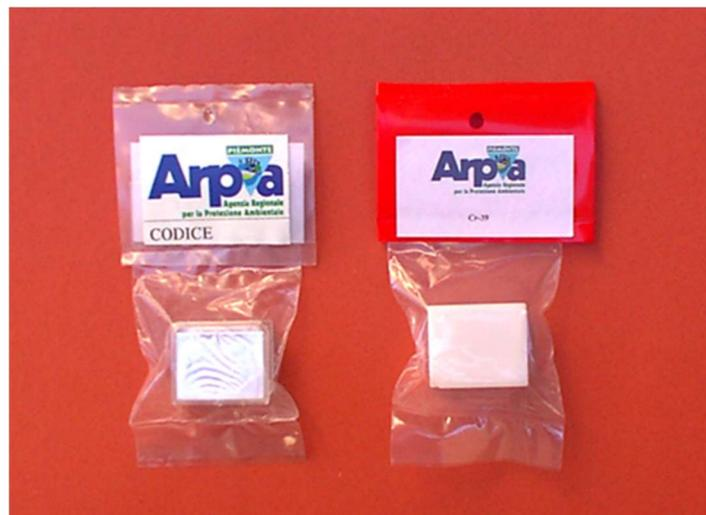
Figure 2 – The ARPA Piemonte dosimeter: radon enters into the dosimeter passing through the radon permeable polyethylene bag
