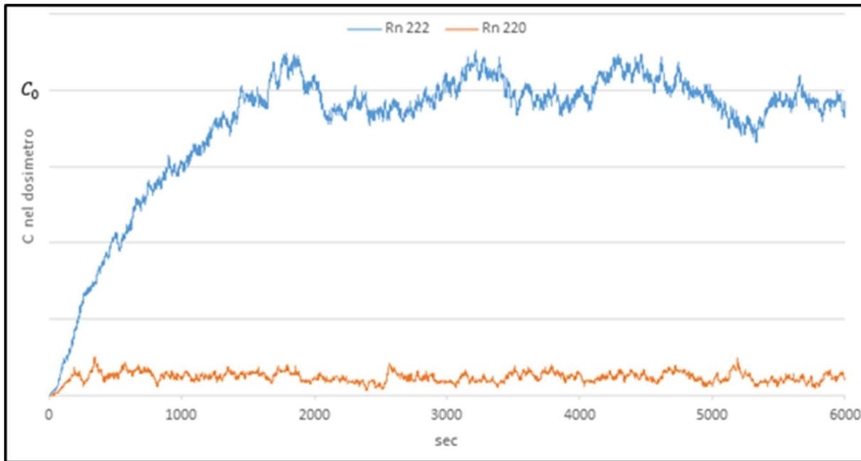
**Figure 5 – Result of the Monte Carlo simulation for radon and thoron. A small but not negligible quantity of thoron enters into the dosimeter**
