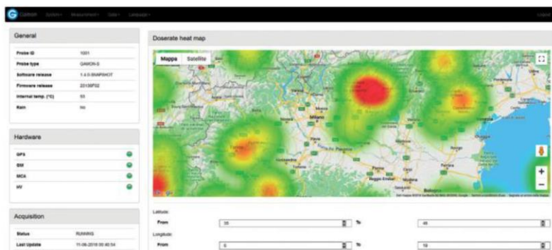
Figure 3: Web page to visualize the count rate, dose rate or isotope presence in the form of a heat map.
