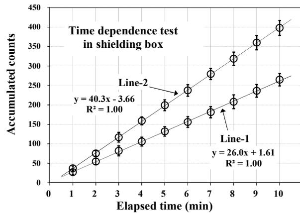
Figure 6: Results of time dependence test carried out in shielding box.
