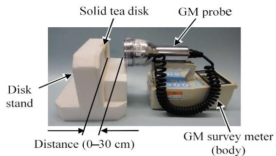
**Figure 1:** Measurement setup of solid tea disk using GM survey meter.
