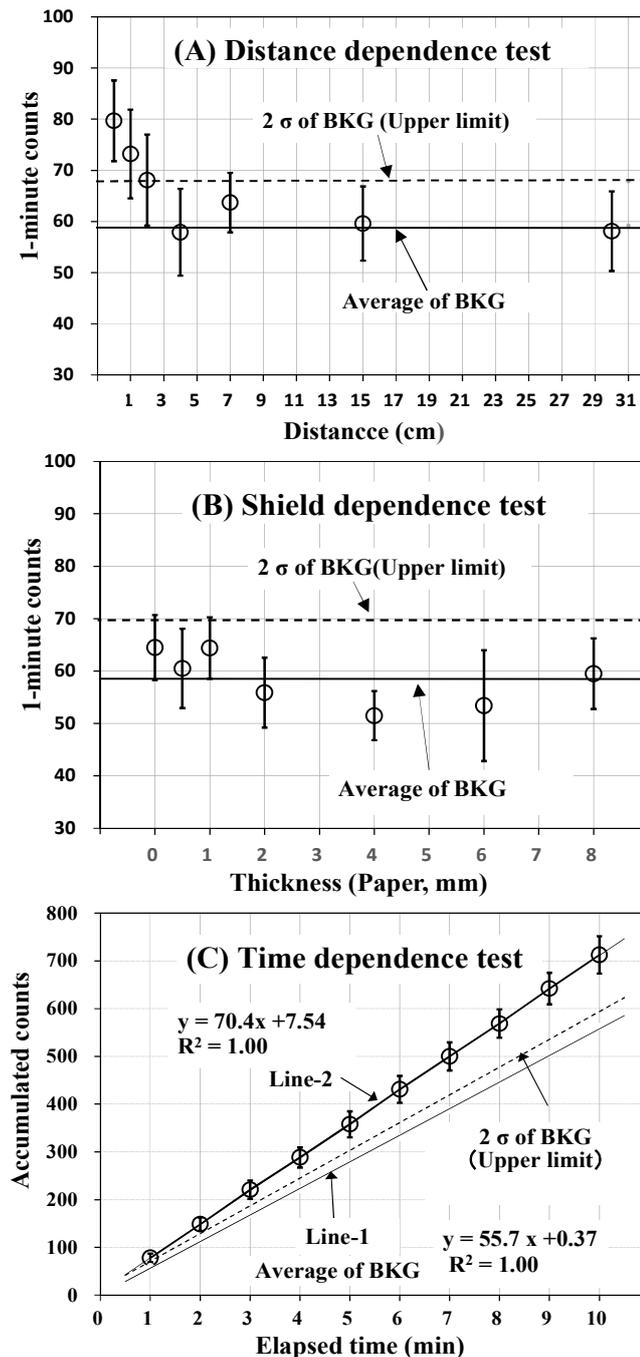
Figure 5: Results of three dependence tests of radiation intensity on distance, shielding, and time.
