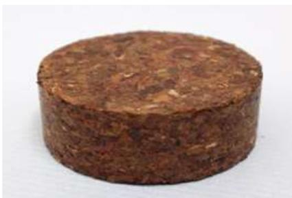
**Figure 2:** Solid disk fabricated from black tea by compression and formation method.
