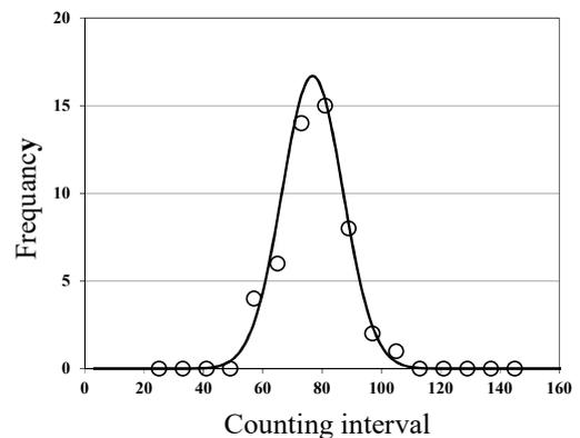
Figure 7: Histogram (frequency graph) and Gaussian curve determined from 1-minute radiation counts for solid tea disk.
