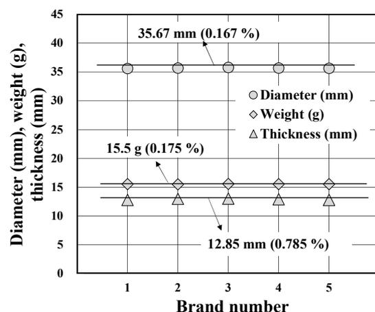
**Figure 3:** Average weight, diameter, and thickness of seven solid tea disks fabricated from five black tea brands.
