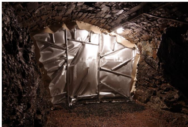
Figure 6: Ventilation experiment in the gallery Silberstrecke with Quick-Erect Stopping System (QESS) set up in the visitor mine Frisch Glück Glöckl in Johanngeorgenstadt [3]
