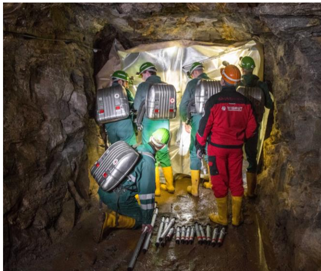
Figure 6: Ventilation experiment in the gallery Silberstrecke with Quick-Erect Stopping System (QESS) set up in the visitor mine Frisch Glück Glöckl in Johanngeorgenstadt [3]
