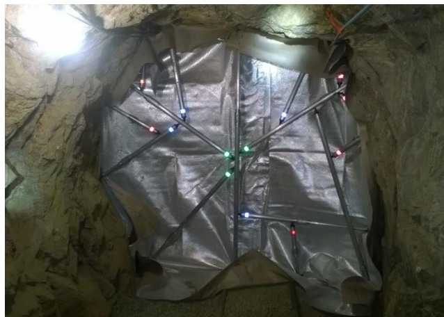
Figure 3: Quick-Erect Stopping System (QESS) in the Edgar Mine, Idaho Springs, Colorado
