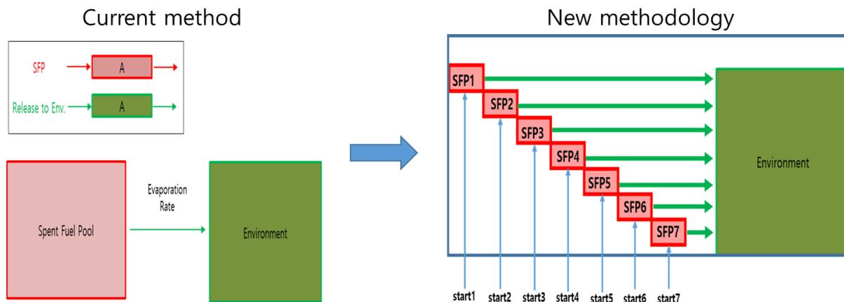
As shown Figure 2, the new RADTRAD methodology has multiple evaporation volumes and the SFP water in each volume is evaporated step-by-step (from SFP1 to SFP7). Each evaporation start time is labeled (i.e., start1, start2, start3, start4, start5, start6, start7).
