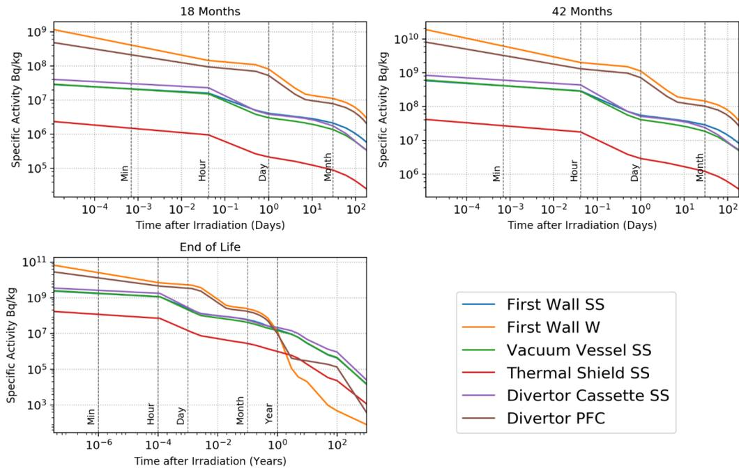
**Figure 5:** DTT contact dose rate from the in-vessel components versus time after irradiation
