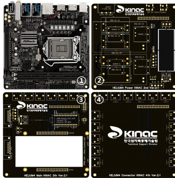
Figure 1. The four boards of the control unit: (1) Windows system board, (2) power supply board, (3) data acquisition layer, and (4) input extension board
