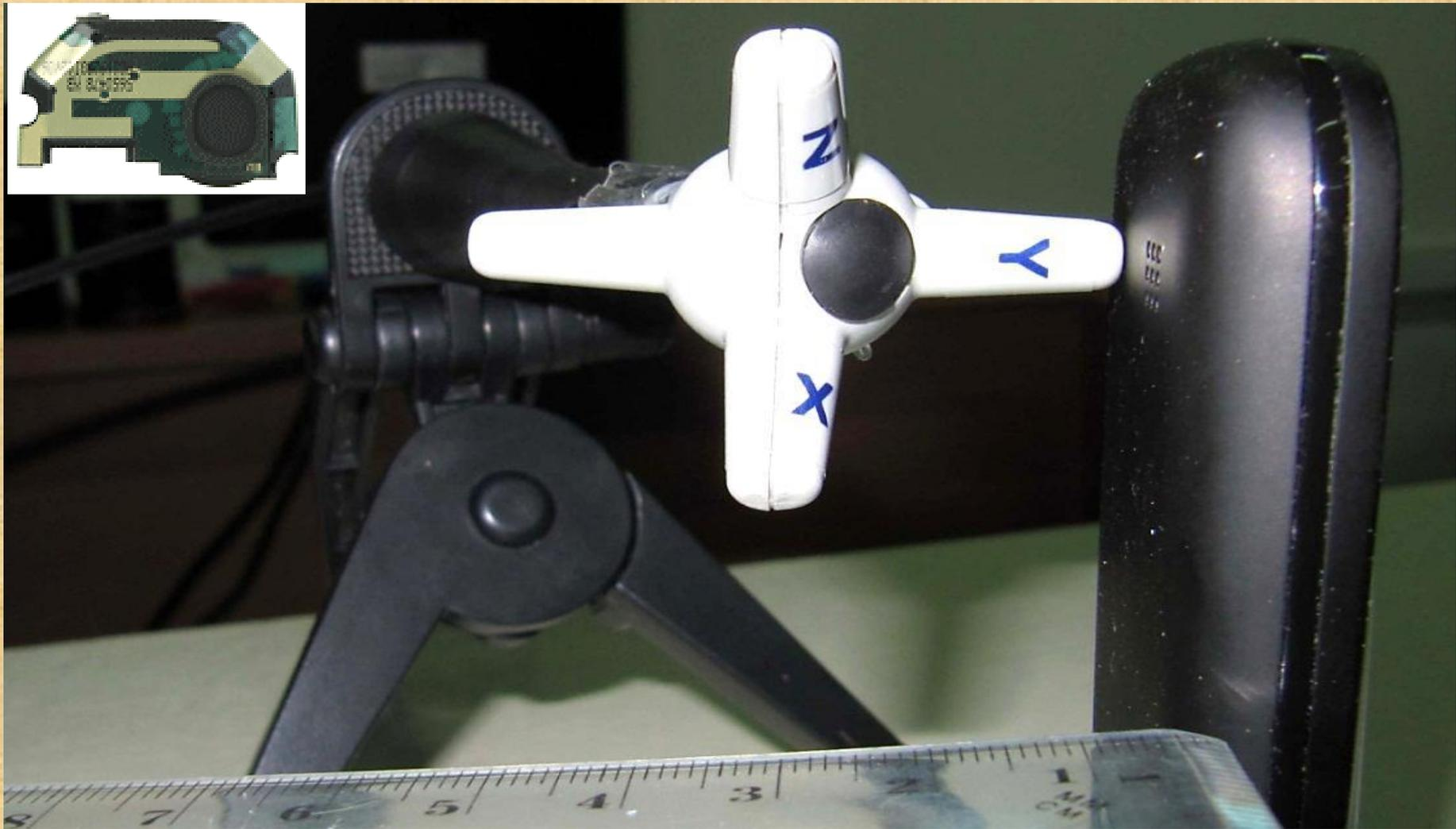
The 3-axis electric field probe at the phone rear, at antenna (inset) height. The antenna is nearer the rear cover and parallel to it
