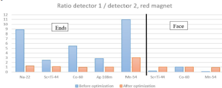
Fig. 2. Ratio between opposite scans activities at the ends and faces of a magnet. A ratio close to 1 shows a satisfactory activity optimization.
