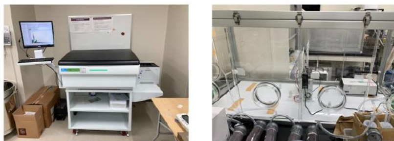
Fig. 1. Liquid scintillation counting system (left) and radon exposure chamber (right).
