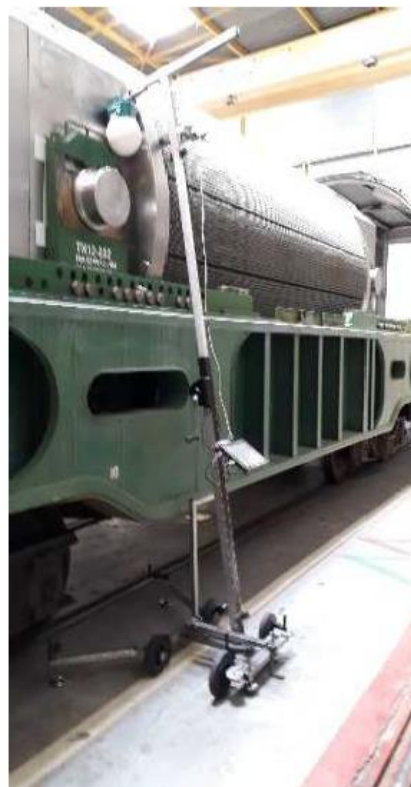
Figure 1. A neutron dose rate measurement at the contact of the cask using the “giraffe” with the PNM200.
