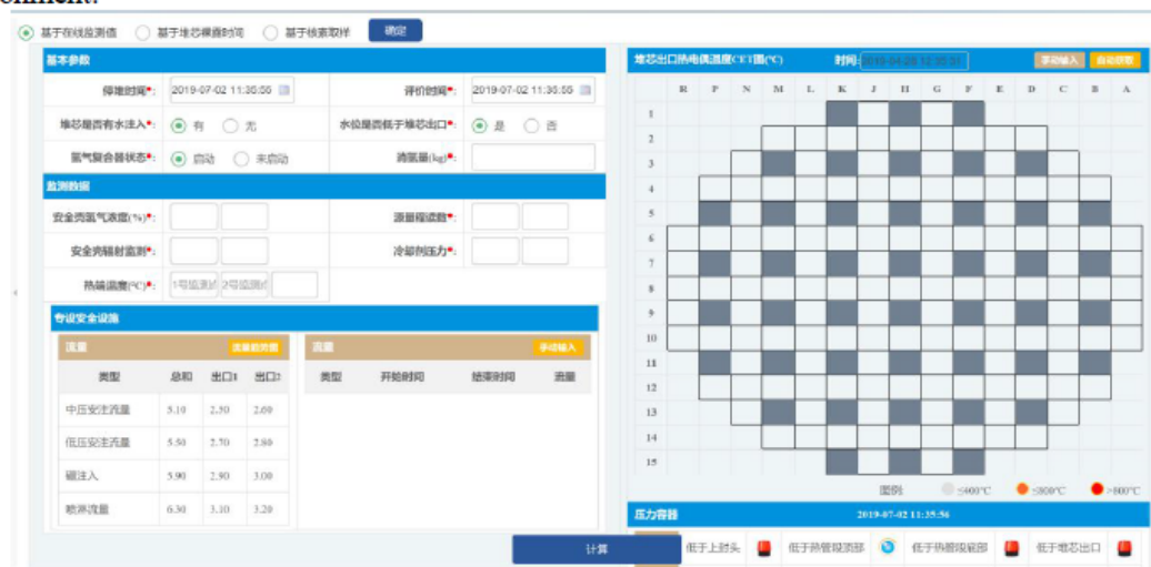
Fig 2. Interface of core damage assessment based on real-time online monitoring instrument readings.
