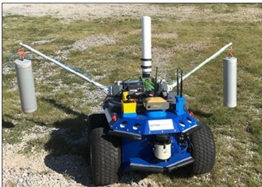
Figure 1 The EPRI robot with LIDAR unit in the front, GPS on the top. Radiation sensors include dual NaI spectrometers on the sides, and a doserate meter.
