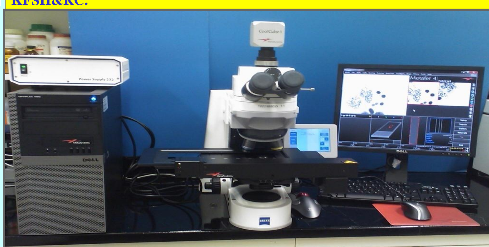
Metafer 4 system for automated dicentric chromosomes scoring installed in the Radiation Biology laboratory at the Biomedical Physics Dept, KFSH&RC.
