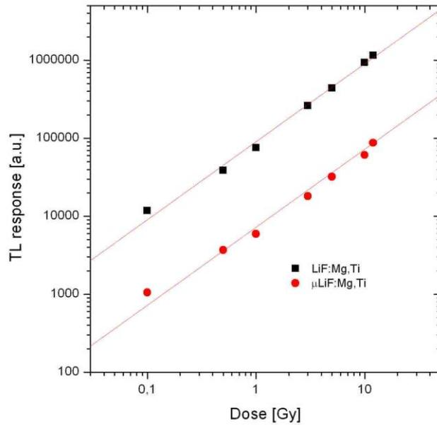
Fig. 1. TL Dose-response curves for the LiF:Mg,Ti and microLiF:Mg,Ti dosimeters.
