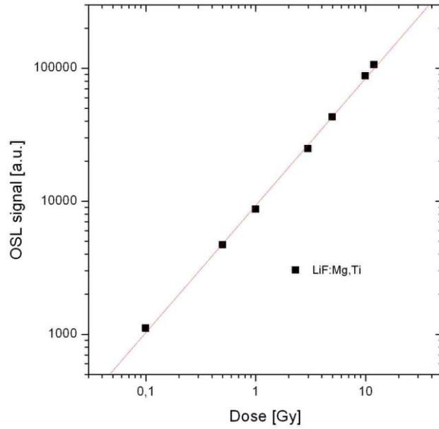
Fig. 2. OSL Dose–response curve for the LiF:Mg,Ti dosimeters.
