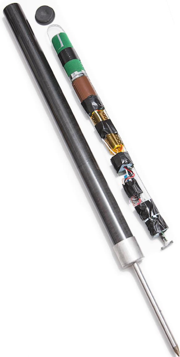
*To simplify transport of the system and to protect it from the elements, it is placed within a water tight carbon fiber tube.*
