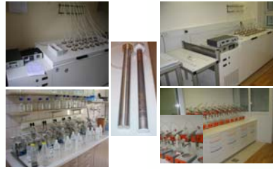
Figure 1. Tritium electrolytic enrichment systems at RBI (left) and IJS (right). In-between: cells for electrolysis.
