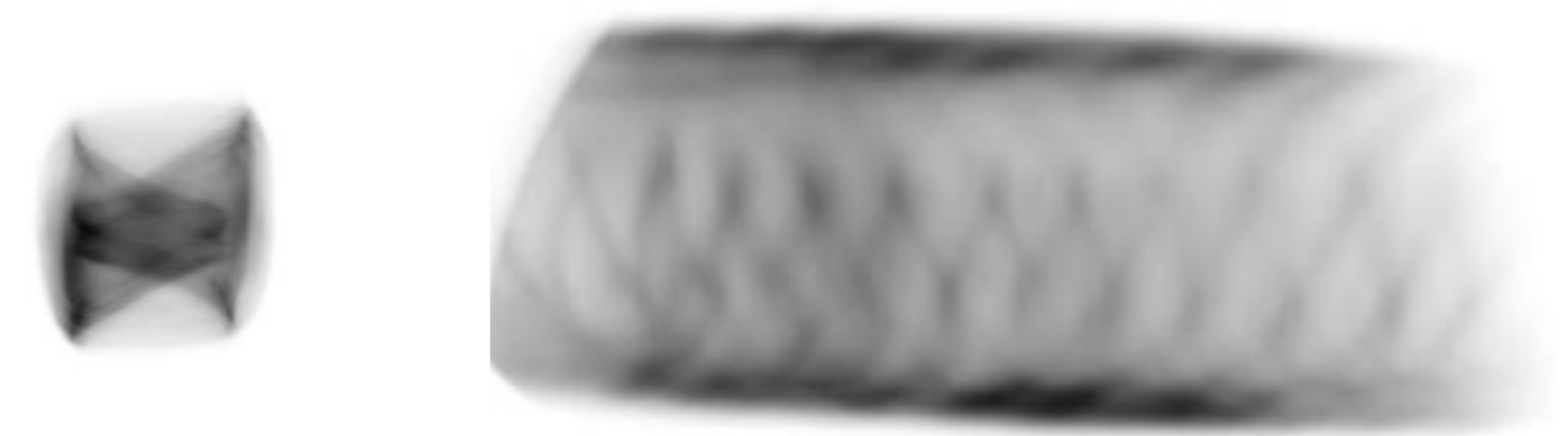
Figure 3: W160 (tungsten X-ray tube) and Mo100 (molybdenum X-ray tube) measured focal spot sizes of about 3.4 mm x 4.3 mm and 12 mm x 5 mm, respectively. A pin-hole collimator was inserted resulting in an inverted and magnified image.
