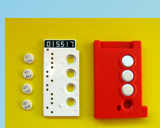
TLD dosimeter type DI-02 and PI-01
