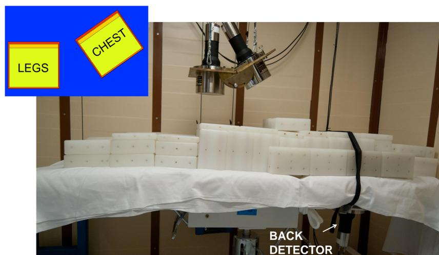
Setup used for the measurement of the IRINA phantom configuration P4. In the left up corner the MCNPX model of the two detectors on top of the stretcher is shown.
