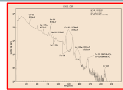
Fig.2 In situ non-destructive measuring gamma spectrometry measured with CZT detector
