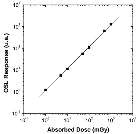
Figure 2 – Dose-response curve of OSL Al<sub>2</sub>O<sub>3</sub>:C detectors exposed to <sup>90</sup>Sr+<sup>90</sup>Y beta standard radiation.
