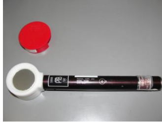
Figure 3. Radcal Ionizing chamber used to test the HVL
