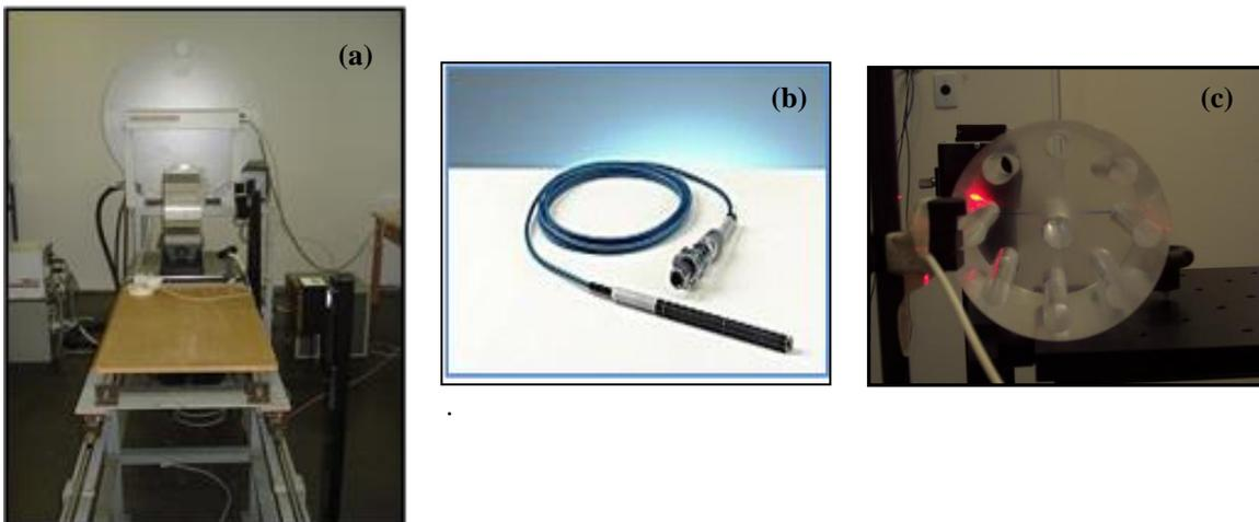
Figure 1: a) ISOVOLT X radiation system (160 kV), b) calibrated pencil ionization chamber; c) pediatric phantom developed by IPEN
