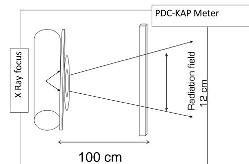
The MCNP5 code was used to calculate the imparted energy in the air cavity of KAP meter and the spatial distribution of the air collision kerma in entrance and exit plans of the KAP meter and on a plane close to the patient. From these data, the air kerma-area product (PKA) and the calibration factor were calculated and its dependencies with the tube voltage, radiation beam size, additional filtration and energy were analyzed.
