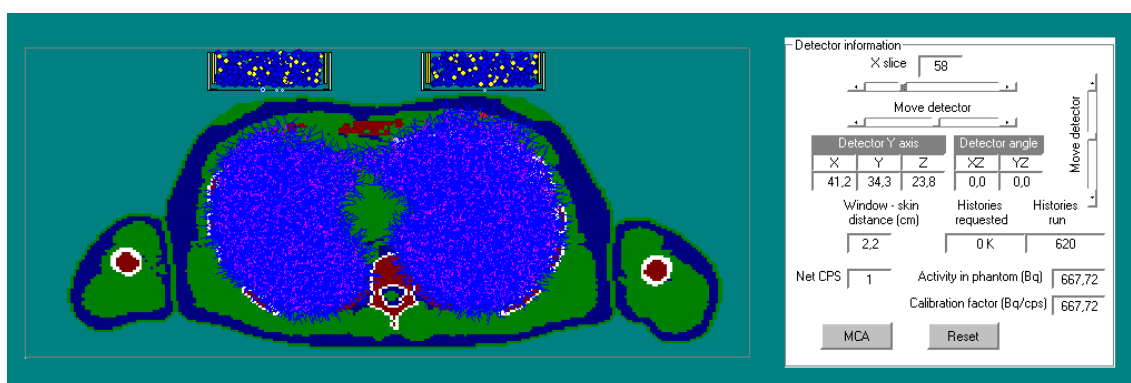
Figure 1. VMC in-vivo simulation of Zr-95 being emitted in the lungs and detected by two BE5030 detectors
