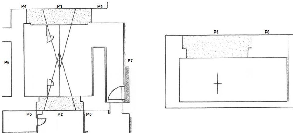
**Figure 1.** On the left: bunker design and identification of the protected points. On the right: vertical section of the installation and identification of the protected points.
