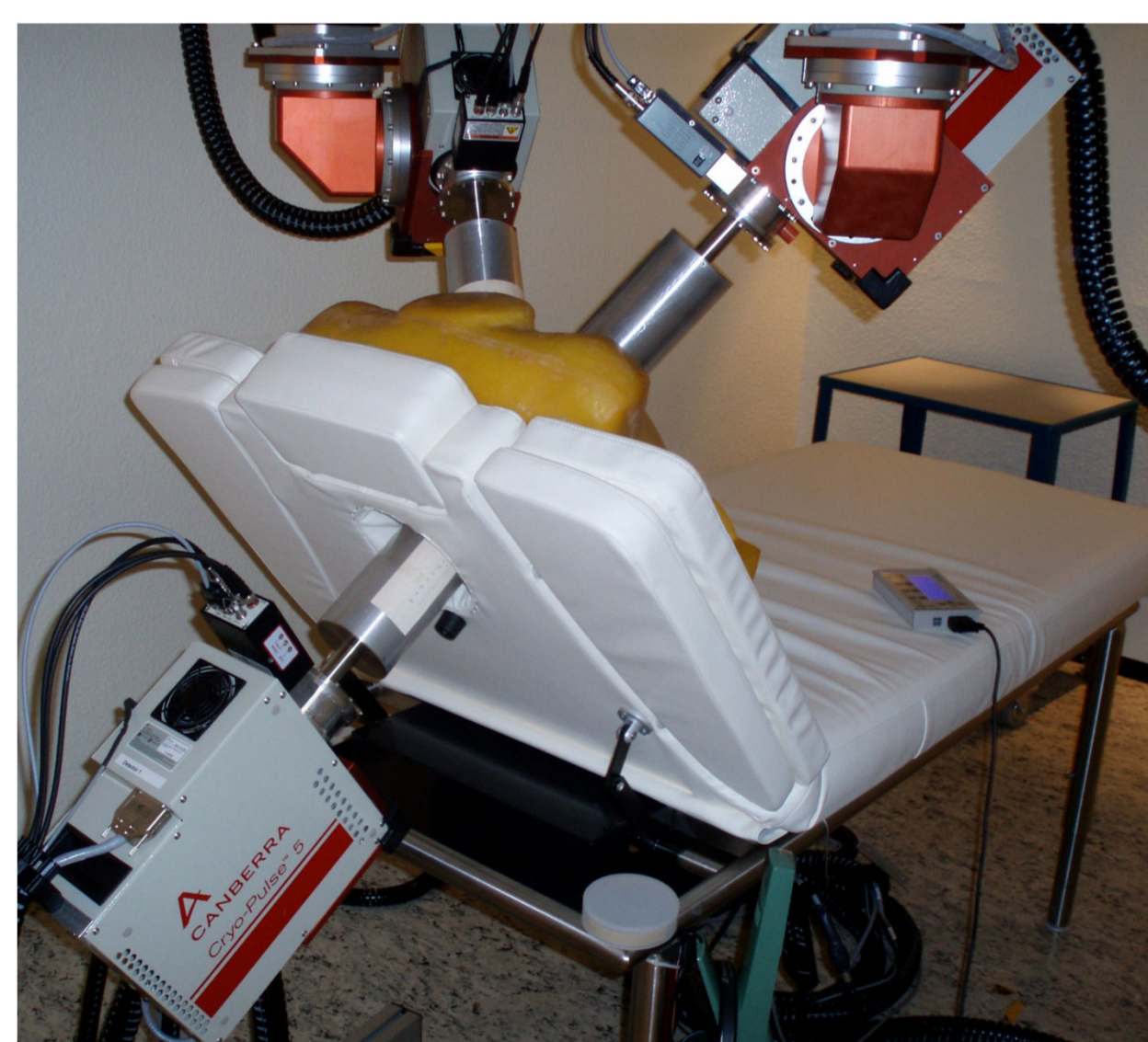
Fig. 1: Exemplary lung counting configuration with physical torso phantom of the local partial body counter.
