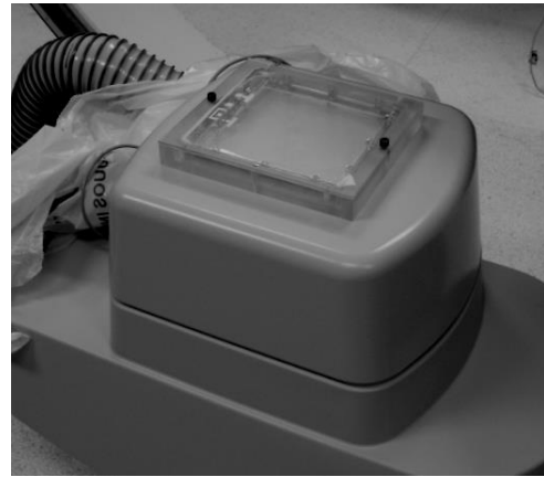
Figure 1. Supports for coupling the chamber to the output of X-ray tube constructed for the equipment.
