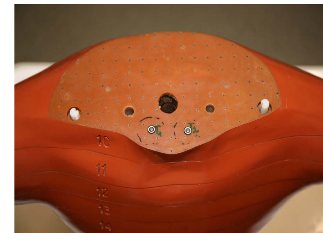
Fig. 3. TLD positions for thyroid glands
