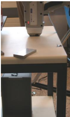
figure 5: primary beam measurement under a table
