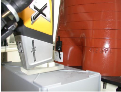
figure 3: scattered radiation on Acrylic glass, XRF tilted
