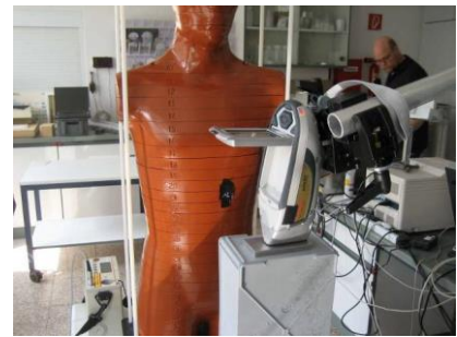
figure 2: measurement with an Alderson phantom
