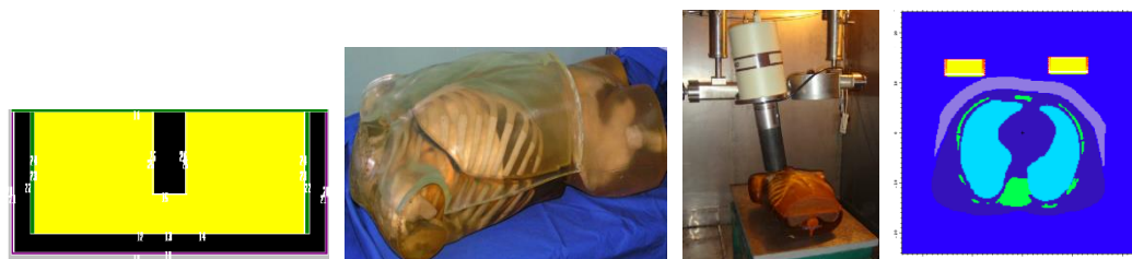
Fig.1 the detector model, CIRP-RPT-1 phantom, the experimental arrangement, the virtual calibration (from left to right)
