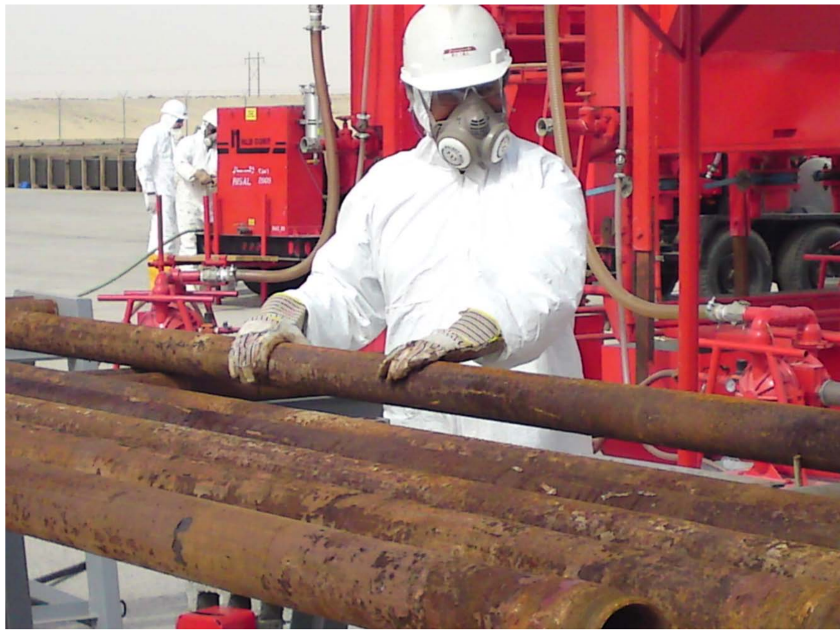
Fig.1. NORM contaminated tubulars.
