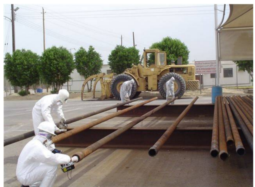
Fig.2. Screening suspect NORM contaminated equipment
