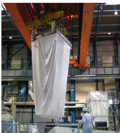
Fig 2. A large tent containing a contaminated component
