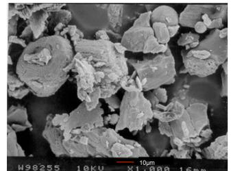
Fig 5. Micrograph of collected dust showing a wide variety of particle sizes
