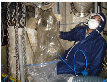
Fig 3. Small isolator in use on the torus
