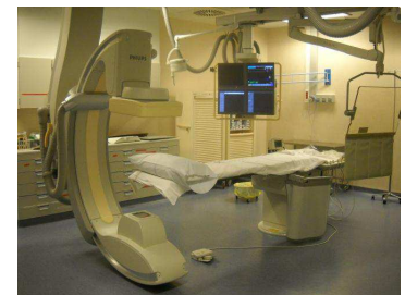
Interventional x-ray unit, equipped with one flat panel
