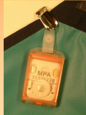
Fig.1: Estimation the effective dose E from single dosimeter measurements assumes an algorithm with the reading either divided by (over-apron case) or multiplied (under-apron case) with a certain correction factor.
