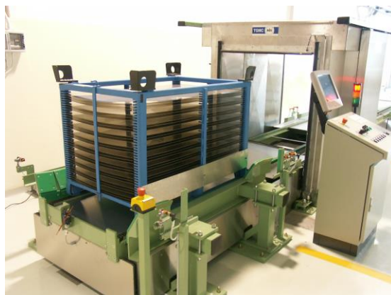
Figure 1 - TGMC system and the standard calibration container
