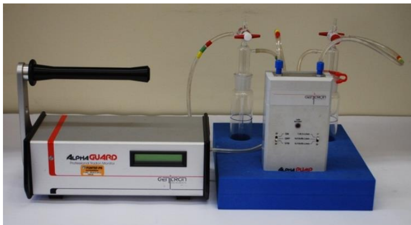
Figure 1. General view of ALPHA GUARD SETTED to measure ^{222}\text{Rn} in well water.
