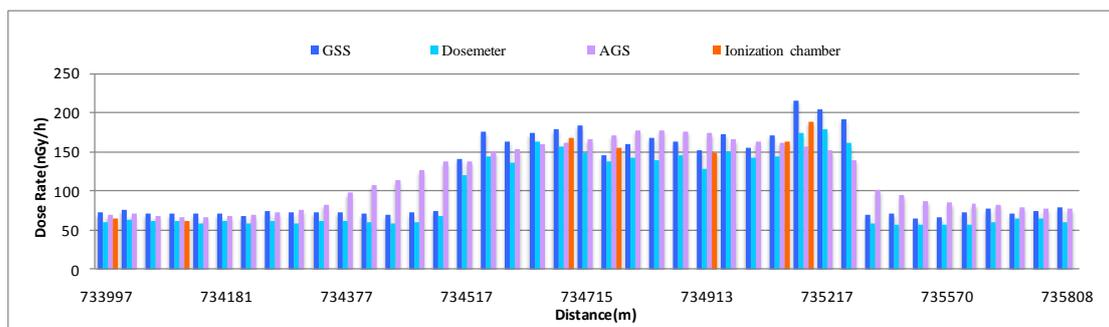
**Fig. 3** Comparison of dose rate by AGS, GGS and a dosimeter
