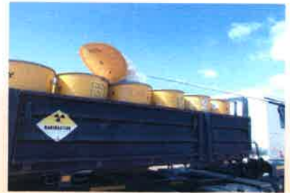
Figure 2. The lid of the waste steel drum came off, the reason was not investigated
