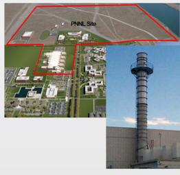
Direct effluent (point source) sampling of the exhaust is typically conducted downstream of the last disturbance and all abatement controls.
